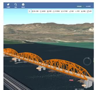
and the IFC standard was integrated into the software and bound with geometric entities to generate the structure objects. To represent the long, linear infrastructure entities, the openBIM model was imported into SuperMap iDesktop, and oblique photography data was superimposed to merge BIM and GIS data.
